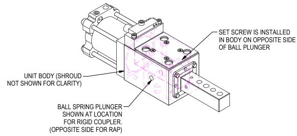
NOTE: IF RAP/RIGID COUPLER IS SWITCHED IN THE FIELD, THE BALL PLUNGER AND SET SCREW MUST BE SWITCHED TO OPPOSITE SIDES.
