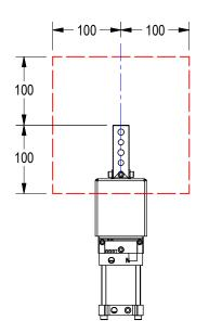
DETENT OPTION EFFECTIVE WEIGHT LIMIT IS 11 LBF FOR VERTICAL APPLICATIONS.
