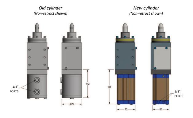
The new cylinder is available with Welker's L3 weld field immune cylinder switch.
