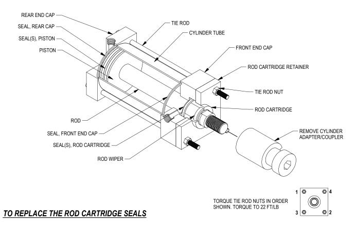
1. Remove cylinder coupler/adapter. Coupler adapter is affixed to cylinder rod with permanent Loctite. To remove, first extend the cylinder rod to move the coupler adapter away from cylinder body. Then apply heat to the coupler to soften the thread locker. Use caution so as not to overheat the cylinder rod seals!
